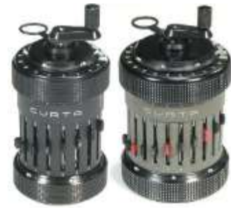
Curta I and Curta II, due to Curt Herzstark (1947)
